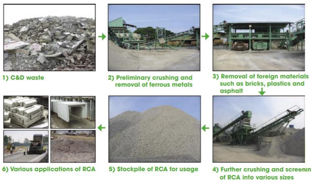
Figure 7: Typical process to reclaim RCA
