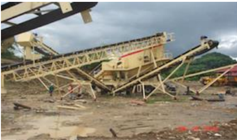
Figure 23: Portable Primary and Secondary Crusher and Screening Plant Delivered for Cavite LGU
