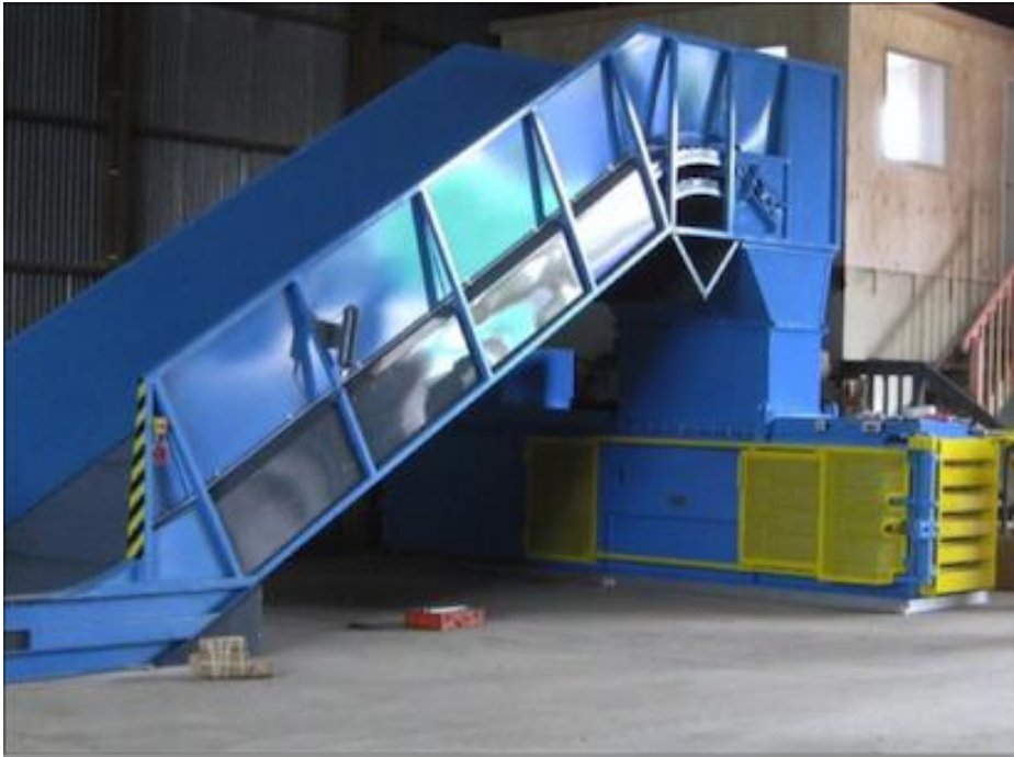
Figure 29: Conveyor Feed from Thai Manufacturer Siam Recycling System
