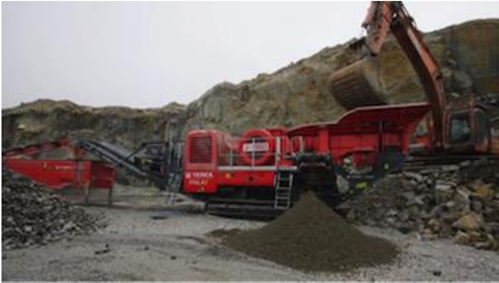
Figure 40: Terex Finlay J-1160 jaw crusher & 684 inclined screen Source: Terex Finlay
